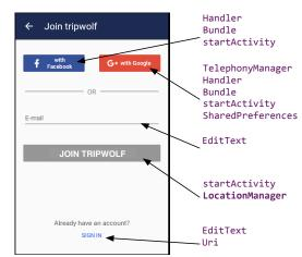
Fig. 1. For each UI element, BACKSTAGE determines the APIs it triggers, and checks for anomalies: The TRIPWOLF Signup button sends the current location to TRIPWOLF servers.
