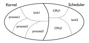
**Figure 3.** The partitioning of the system state enforced by the logic. The memory is partitioned into two parts, owned by the scheduler and the kernel, respectively. The memory of each component is further partitioned into parts local to processes or scheduler invocations on a given CPU, and parts protected by locks.
