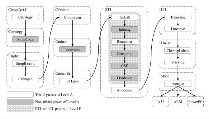
Figure 9. Optimization passes of SepCompCert Level A and Level B.
