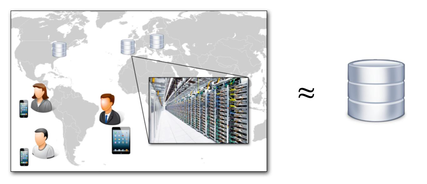
Strong consistency model: the system behaves as if it processes requests serially on a centralised database
