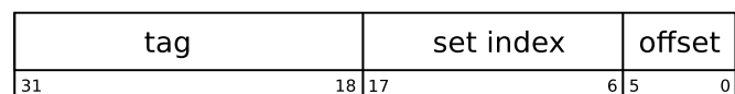
Figure 4.1: An example split of a 32-bit memory address into tag, index, and offset, for a physically indexed and tagged, 32KB, 8-way set associative cache, with 64-byte lines.
