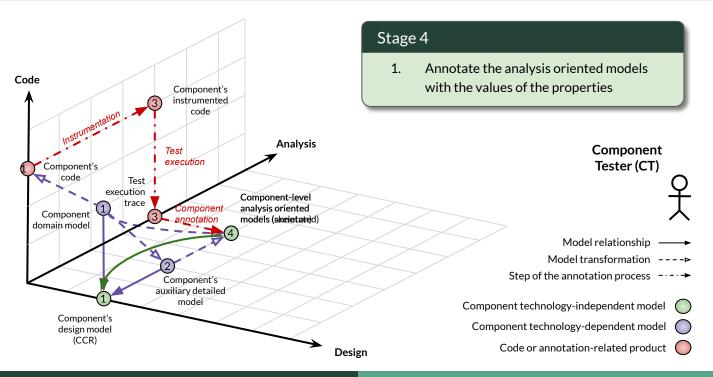
**Component model and analysis tool integration** System-level analysis of the application software of EPD's ICU
