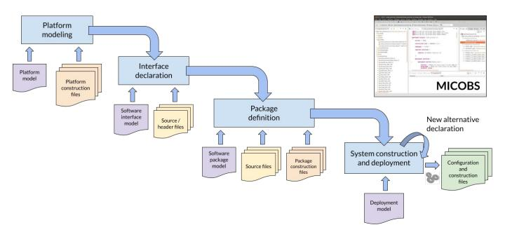
Component model and analysis tool integration system-level analysis of the application software of EPD's ICU
