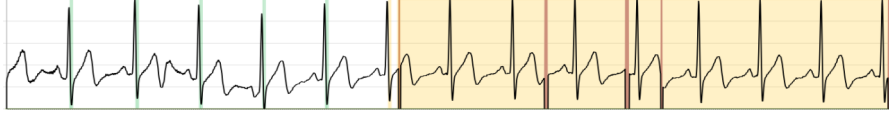
Figure ECG analysis with 5 bursts of fully uncertain values(5 to 20 in a row). Interval approach. Orange: Burst of uncertain values; green: heartbeat certainly detected; yellow: heartbeat possibly detected.
