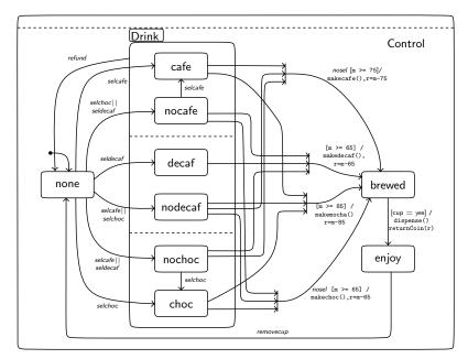
Fig. 3: Statechart for a CVM without state explosion.
