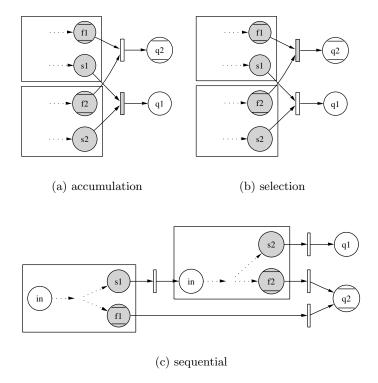
**Fig. 4.** Correlation modules for accumulation, selection and sequential. The shaded circles denote the success and failure nodes of the modules  $\mathcal{M}_{\{1,2\}}$ , and the unshaded circles denote the success and failure nodes of the resulting module. Transitions with conjunctive enabling condition are shown shaded and disjunctive transitions are unshaded.
